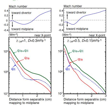
"near-SOL" e-folding lengths of el. & total heat flux profiles for 4 cases of  $P_{\text{sep}} \& f^*_{\text{rad}}^{\text{div}}$
