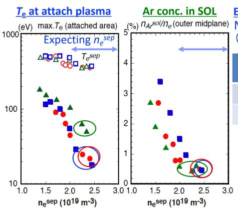
Ar conc. in SOL Estimation of net-erosion with 90% re-deposition Net erosion ( $\triangle d$ ) becomes a half of W-width (d:5mm), if  $T_e^{\text{div}} \sim 20 \text{eV}$  at attached area.
